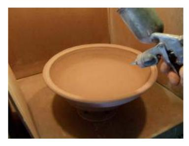
Now let's look at how the glazes are applied. In this picture, the underside of a platter rim has already been sprayed. The platter has been turned over, right side up, and a measured quantity of chocolate glaze is being sprayed evenly on the top.
