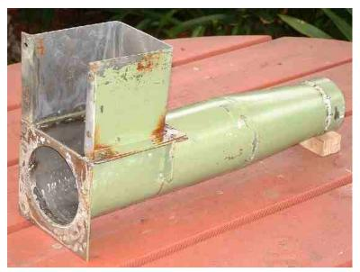
The hopper is a simple folded box made up from lighter gauge stainless sheet., fixed to the main barrel with six small bolts. The rusty stains are from these bolts, sold as "stainless" but they corroded anyway.
