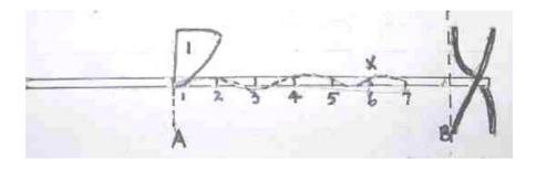
Make 2 turns between A and X so blade 6 will fit on the shaft in the same position as blade 1. Trace this spiral onto the shaft with a felt pen. The intersections of the spiral path and the circular bands 2 to 7 give the contact points of blades 2 to 7
