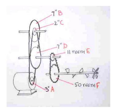
The speed reduction in this model was done using vee belts and pulleys, then a chain and sprocket drive to the auger. Pulley A on the motor (3 inch) drives pulley B (7 inch) on a layshaft. Then C drives D, on a second layshaft which also carries a toothed sprocket E (11 teeth)
