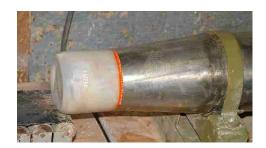
Unless the finished pugmill is used almost every day, its contents are likely to dry out. You can delay this by providing a plastic cap over the delivery end, as in this picture.
