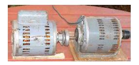
This photo shows two motors salvaged from old washing machines. The one on the left, with the extra cylindrical thing stuck on the top, is a "capacitor start" motor. It has the useful property of developing a high torque from a standing start. In other words, it's designed to start under load, which is what you want in a pugmill.
