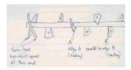
This photo shows one of the long-ago sketches made when building the first pugmill. Blades 1 to 7 resemble a continuous single spiral of pitch approx 150 mm, with alternate sections removed. One revolution of the spiral occupies about 150 mm.
