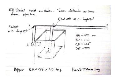
The left end of the long handle was welded rigidly to a further short bar, descending to the only hinged joint in the whole construction, at A (lower left of sketch). One would think that the descending plunger would bind against the hopper wall, but there was enough clearance for it to move. I chose to make mine with a closer fit between plunger and hopper, but this required
